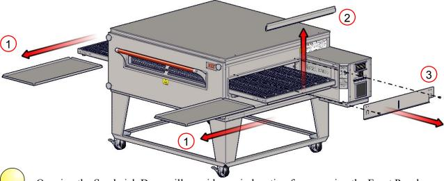
Opening the Sandwich Door will provide a grip location for removing the Front Panel.
