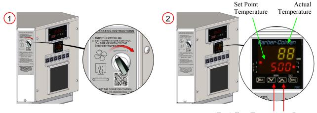
To Adjust Temperature Press Either the Up or Down Arrow.
