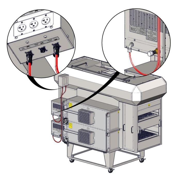
All hoods are outfitted with three (3) switch relocation outlets, regardless of how many XLT Ovens are installed. For a single oven use "Top" location. For a double stack use "Top" location for upper oven and "Bottom" location for lower oven, leaving "Middle" location open.
