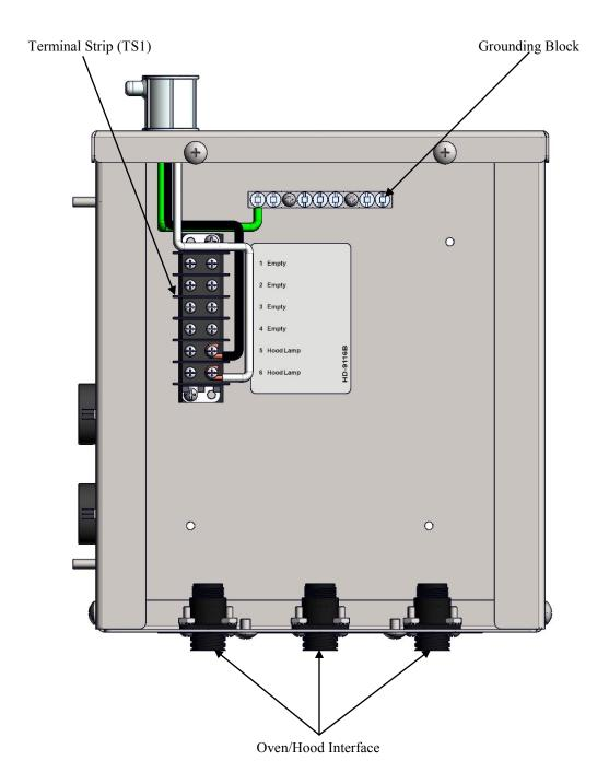
Non-VFD Control Box (Cover removed)
