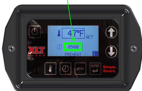
③ **BELT TIME ADJUST:** Press TIME button for three (3) seconds. To adjust belt time use either the Up or Down arrow until desired belt time is displayed and then press Enter
