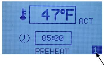
The Menu programming can store up to twelve (12) preset menus that can be recalled by number as needed. Each program contains a specified baking temperature and belt time.
