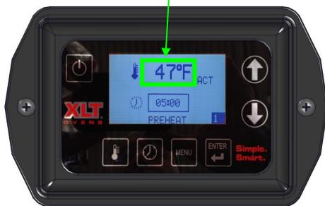
② **TEMPERATURE ADJUST:** Press TEMP button for three (3) seconds. To adjust temperature use either the Up or Down arrow until desired temperature is displayed and then press Enter
