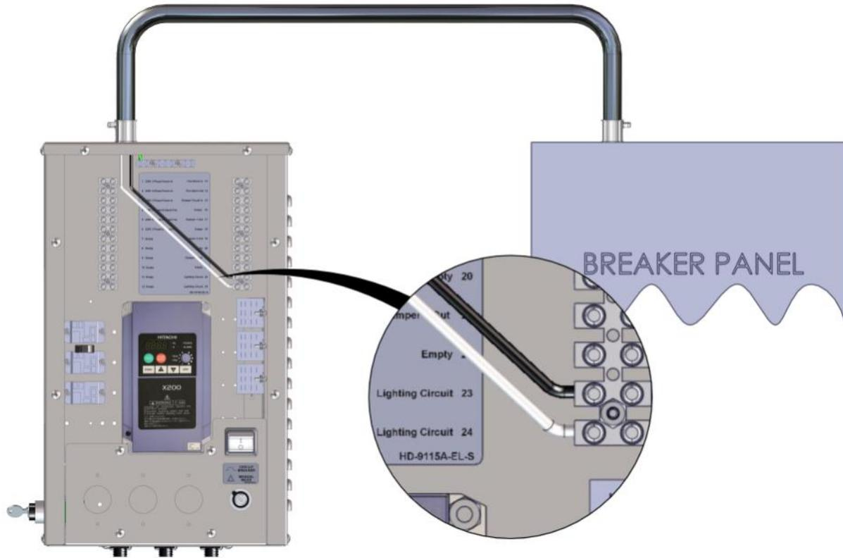
Power from VFD to Exhaust Fan - Standard Voltage & Frequency
