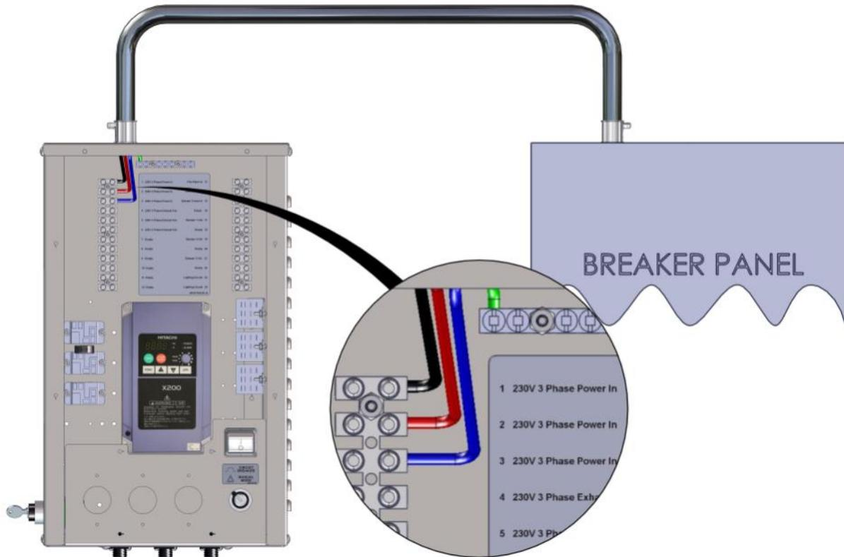
Input Power to Lights with VFD- Standard Voltage & Frequency
