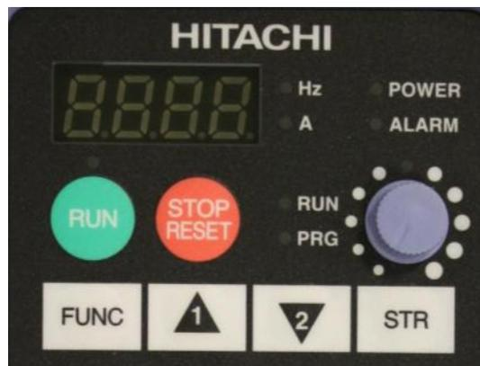
Put controller into monitor mode by pressing the <FUNC> and holding until d001 appears on the display release and then press the <FUNC> one time. The display should show 0.0.
