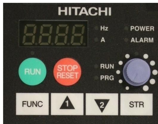
Put controller into display mode by pressing the <FUNC> button and holding until d001 appears on the display release and then press the <FUNC> button one time. The display should show 0.0.
