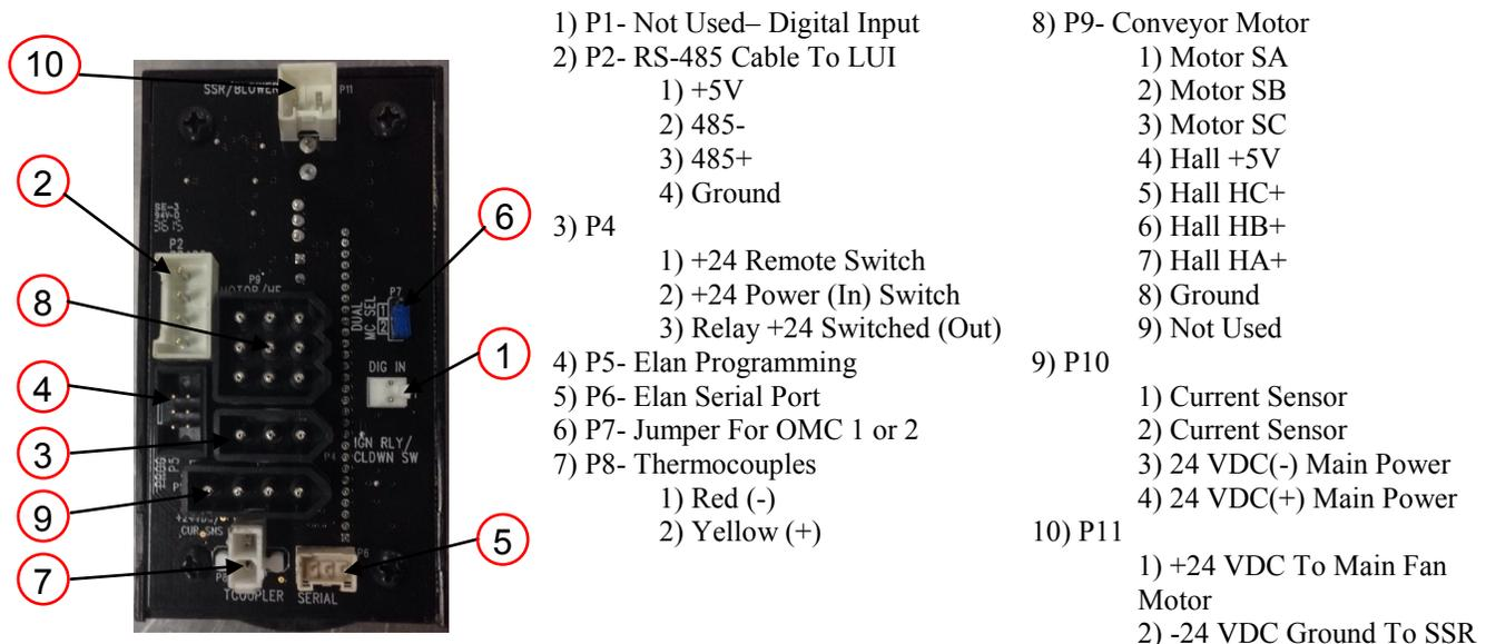
**OMC** - The Oven Machine Control reads selections or parameters from the LUI. It holds the logic for the conveyor controls and the temperature controls. The OMC will turn on or off SSR’s, start and stop M1, send the call for heat signal, reads the thermocouple and monitor the current sensor.
