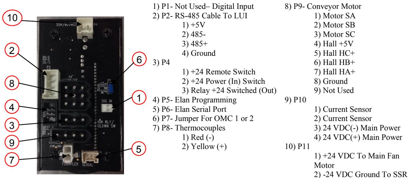
**OMC** - The Oven Control reads selections or parameters from the LUI. It holds the logic for the conveyor controls and the temperature controls. The OMC will turn on or off SSR’s, start and stop M1, send the call for heat signal, reads the thermocouple and monitor the current sensor.
