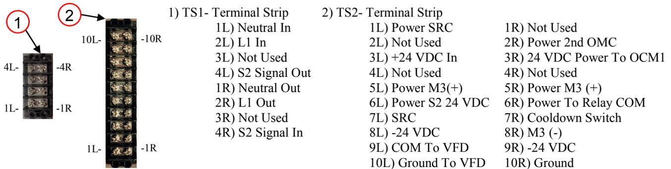
**TS 1 & 2-** These are terminal strips, that serve as a connection point for wires.
