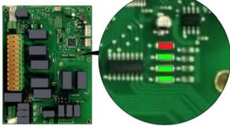
1. When the Red LED is lit it indicates an MC error.
