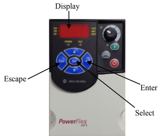
With the Oven Control switched off and power connected to the oven, the VFD should show 0.0 on the display.
