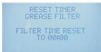
1. The Cooling Fan and Grease Filter reset alarm will show up in the lower left hand side of the Hood User Interface. Press the Error Information button to enter reset screen.
