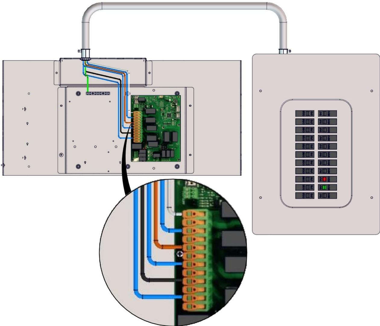
Input Power to VFD Controller - Standard (120V / 60Hz)
