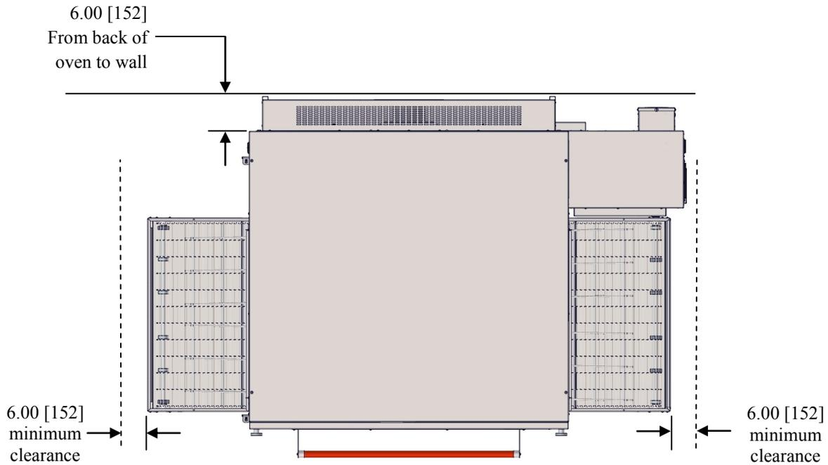
**NOTE** Utilities must be easily accessible when the ovens are in the installed position. Do not install utilities behind the ovens.
