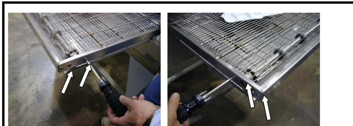
Tension the belt and replace the four (4) screws removed earlier from the idler/tension shaft blocks.
