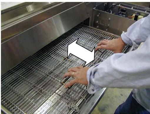
Check the conveyor belt for free movement.
