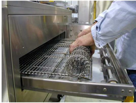
Roll the fabric carefully as shown. Do not crimp, fold, or roll tightly.
