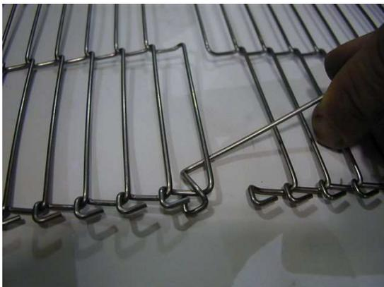
Pass the hook back around the wire until disengaged.
