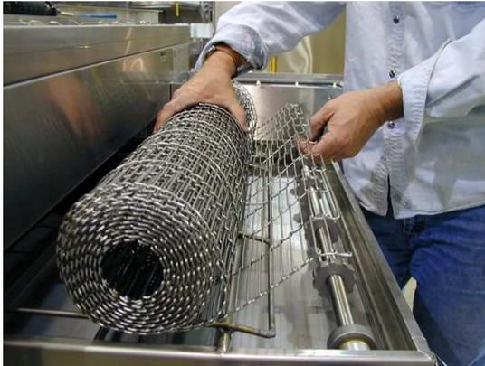
Once rolled, turn the fabric end-for-end in preparation of reinstallation.
