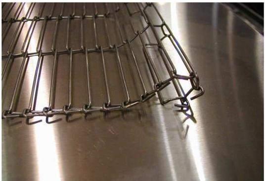
Fabric orientation is critical for the service life of the belt. Check to see that the correct side is up by curling the end as shown.
