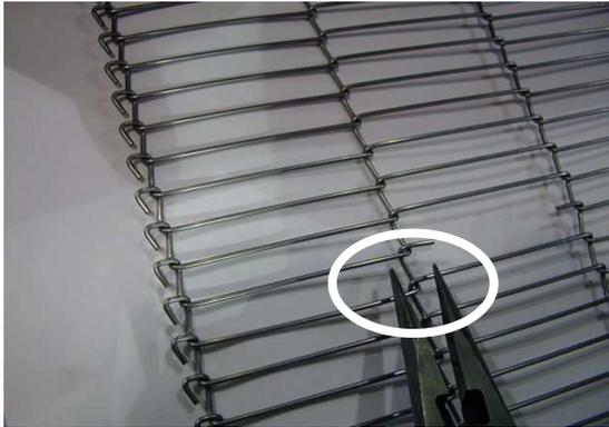
Using a pair of needle-nose pliers, grip the free end of the first splice link.
