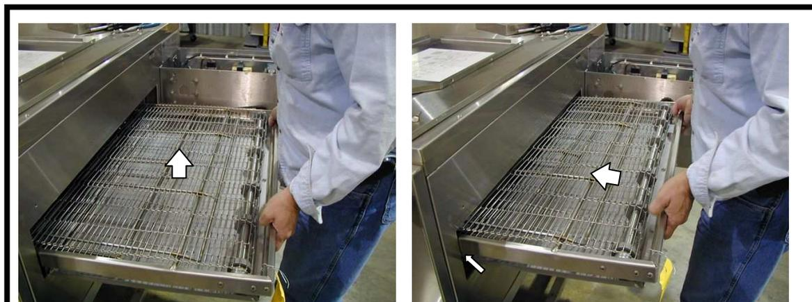
Grasp the conveyor firmly and lift up until the crumb tray bracket clears the conveyor opening. Slide the conveyor 1" – 2" into the oven to release the tension on the chain.
