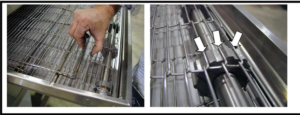
The belt is ready to be re-connected at the splice joint. The process for this connection is simply the reverse of the process described earlier during disassembly. Once the belt has been spliced, check the alignment of the power and idler sprockets for proper engagement as shown.
