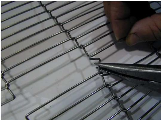
Care should be taken to keep from distorting the splice links during removal. Set aside all links for reuse.
