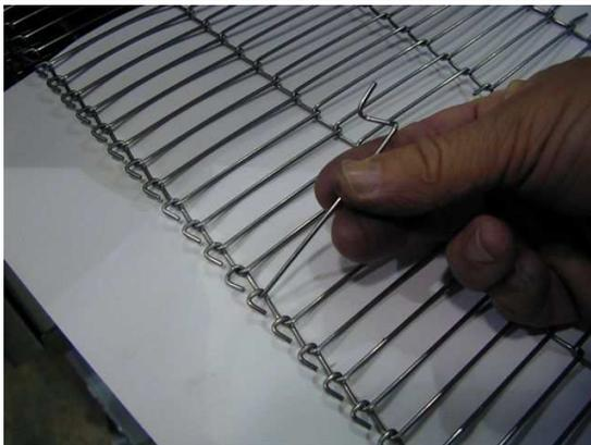
To release the edge link, rotate the link up as shown ...
