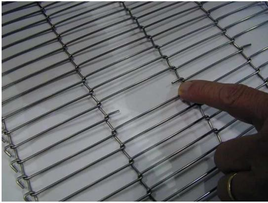
Find the belt splice by manually advancing the fabric.
