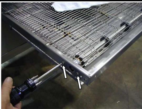
Release belt tension by removing two (2) screws each at the idler/tension shaft blocks.
