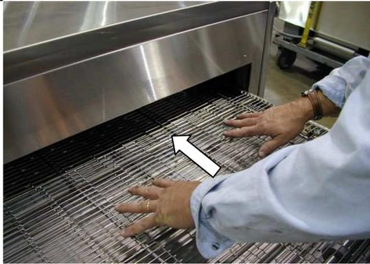
As you reach the idler sprockets, feed the belt from underneath, over the sprockets across the upper conveyor surface and back through the remaining conveyor belt circuit.
