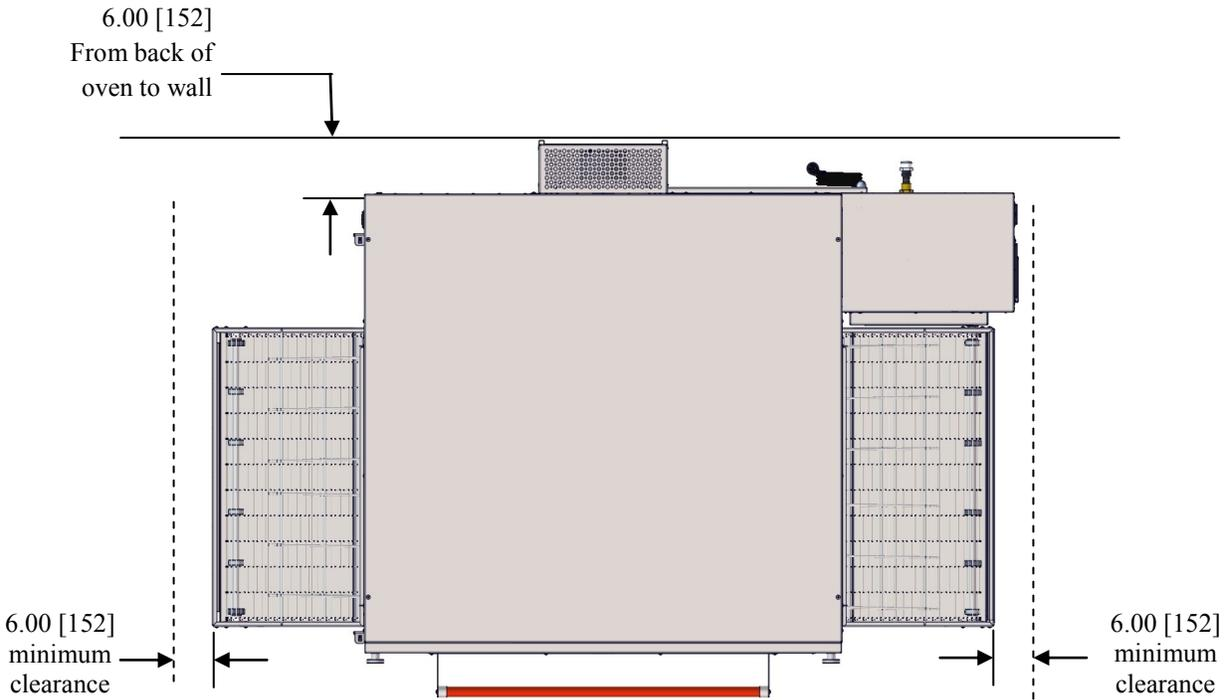
**NOTE** Utilities must be easily accessible when the ovens are in the installed position. Do not install utilities behind the ovens.
