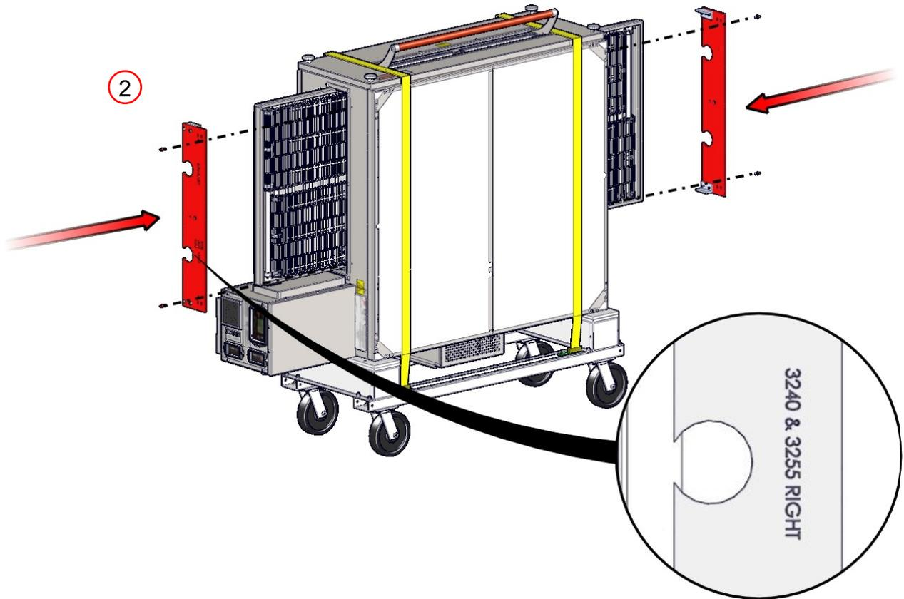
**NOTE** → The Lifting Pipe hole, marked for the appropriate oven size, must be installed closest to the control box.
