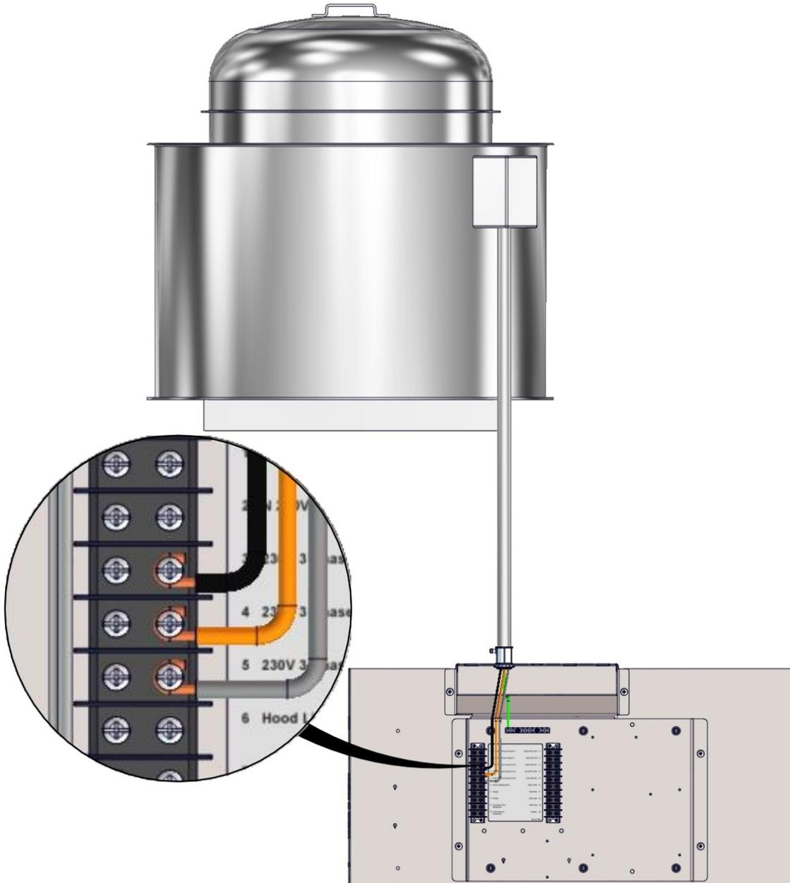
MUA Damper Relays - Single Output - Voltage & Frequency
