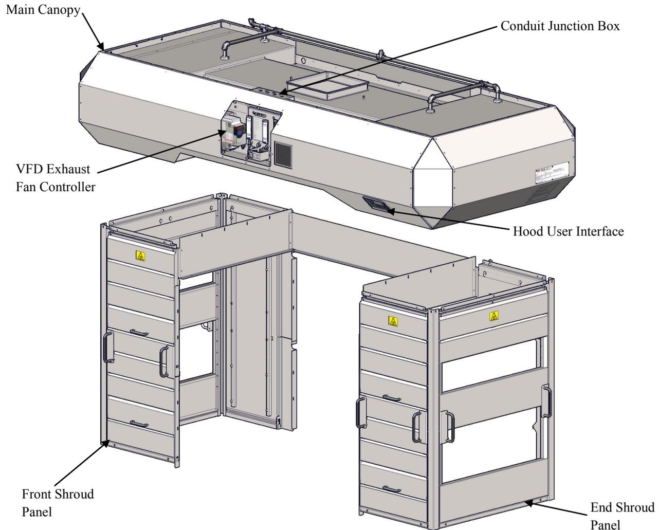
The AVI Hood System consists of three (3) major parts; the Main Canopy, the Shrouds, and the Variable Frequency Drive (VFD) exhaust fan controller.
