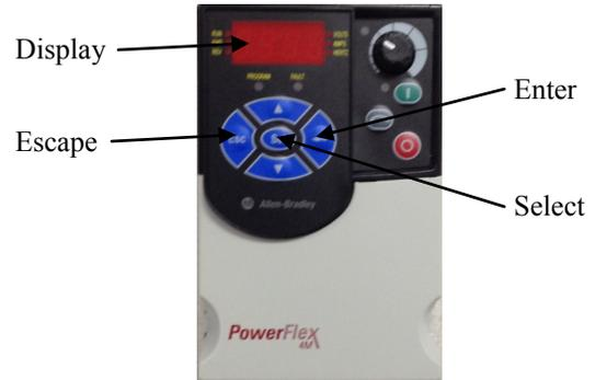
With the Oven Control switched off and power connected to the oven, the VFD should show 0.0 on the display.
