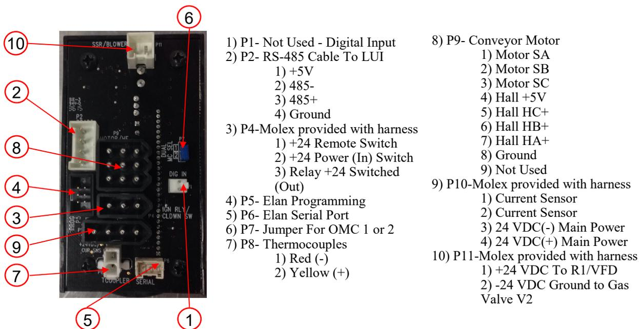
**OMC** - The Oven Machine Control reads selections or parameters from the LUI. It holds the logic for the conveyor controls and the temperature controls. The OMC will turn on or off SSR's, start and stop M1, send the call for heat signal, reads the thermocouple and monitor the current sensor.
