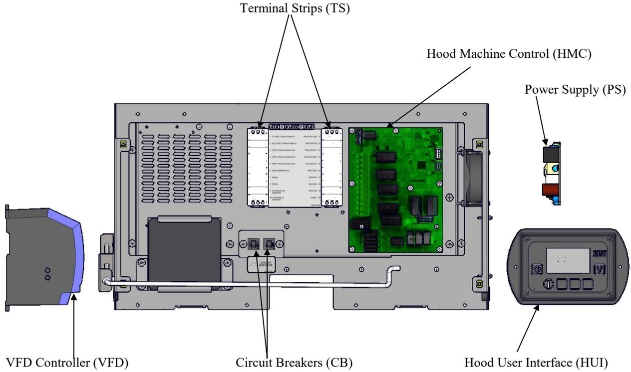
VFD Control Box (Cover removed)
