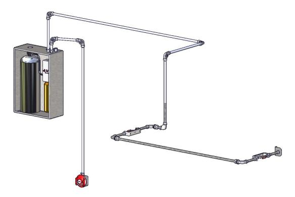
4. Install a fusible link with temperature rating of 360°F (182°C) to the scissor style linkage at each detector. These are located on the ends of the hood.
