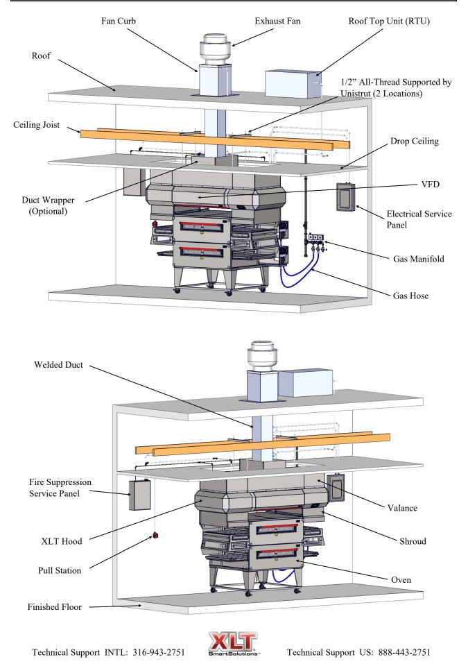
The Engineers at XLT have designed the fire suppression system for XLT ovens and XLT hoods to meet ICC and NFPA codes. Field installations can be more expensive, less effective, and can interfere with daily operations and maintenance.
